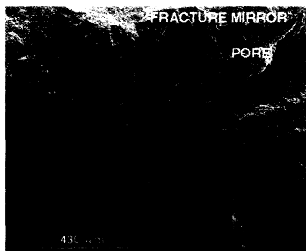
Fig. 5. Typical fracture-initiating flaw in Si-SiC measured in fast-fracture at 1400°C.
